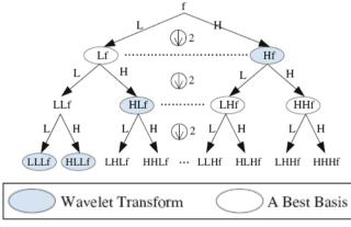
Fig. 1. Illustration of the wavelet packet decomposition.
