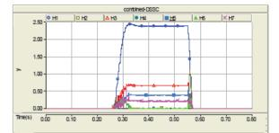
Fig. 10. harmonics of the injected voltage by combined-DSSC
