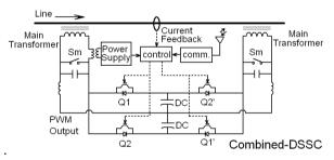
Fig. 4. circuit schematic of combined-DSSC module
