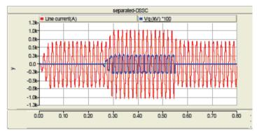
Fig. 7. The current in one phase and the injected voltage Vq by the separated-DSSC module
