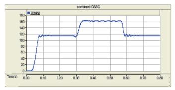
Fig. 6. transmission reactive power for combined-DSSC module
