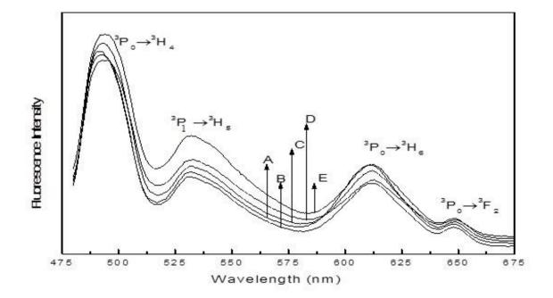
Fig.2. Emission spectra of Pr<sup>3+</sup>: BZCAP 1-5 glasses
