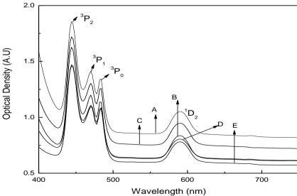
Fig-1 (a) Optical absorption spectra of Pr<sup>3+</sup>: BZCAP 1-5 glasses
