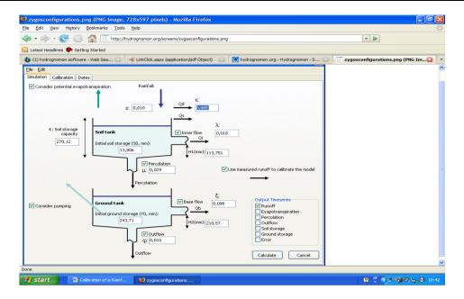
Fig 2 Structure of the Simulation module (http://www.hydrognomon.org)
