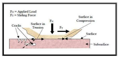
Schematic of fatigue wear, due to the formation of surface and subsurface cracks.
