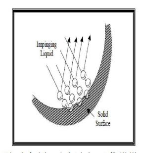
Schematic of cavitation erosion due to impingement of liquid bubbles.
