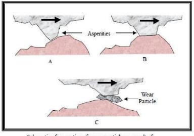
Schematic of generation of a wear particle as a result of adhesive wear process. Fig 5 Adhesive Wear
