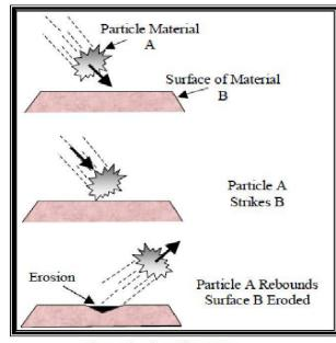
Schematic of erosive wear. Fig 3. Abrasive Wear due to solid erosion
