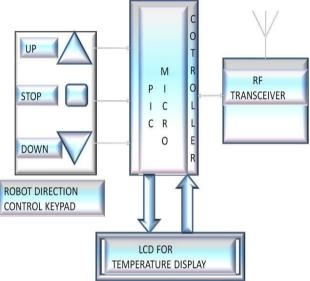
Fig. 5: Direction controller Handset Block diagram
