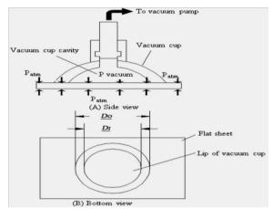
Fig. 1: Vacuum cup used to lift a flat sheet
