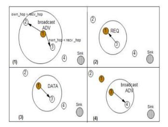
Figure 4. The M-SPIN protocol. (1) Node 1 starts advertising its data to all of its neighbors. (2) Node 3 responds by sending a request to node 1. (3) After receiving the request, node 1 sends the data. (4) Node 3 again sends advertisement out to its neighbors for the data that it received from node 1.
