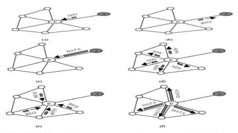
Figure 3: The SPIN-BC Protocol. Node A starts by advertising its data to node B (a). Node B responds by sending a request to node A (b). After receiving the requested data (c), node B then sends out advertisements to its neighbors (d), who in turn send requests back to B (e,f).
