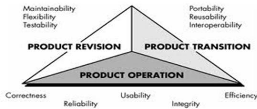
Figure 1: The McCall quality model (a.k.a. McCall’s Triangle of Quality) organized around three types of quality characteristics.
