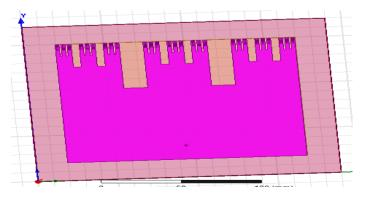
Fig.3, the pictorial representation of the proposed design for third iteration of E-shape fractal (3EFPA) is produced with optimized dimensions.
