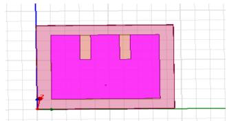
Fig.1, the pictorial representation of the proposed design for first iteration of E-shape fractal (1EFPA) is produced with optimized dimensions
