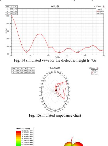
Fig. 16 simulated gain with the value of gain = 8.3db
