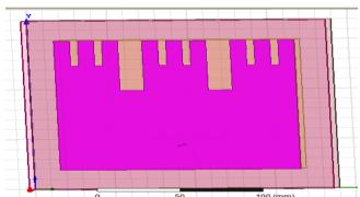
Fig.2, the pictorial representation of the proposed design for second iteration of E-shape fractal (2EFPA) is produced with optimized dimensions
