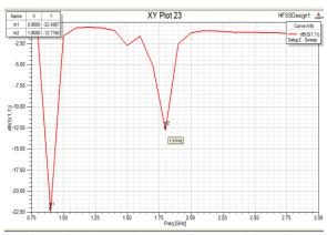
Fig. 9 simulated return loss for second iteration.
