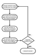
Fig. 2. Flow diagram outlining the procedure for using the Levenberg- Marquardt training algorithm
