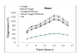
Fig. 6, Various target temperatures variations with time on June
