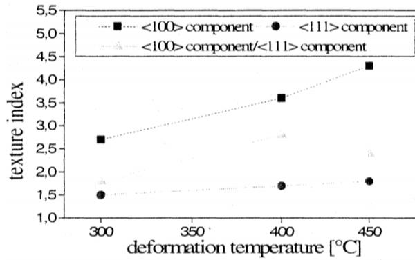
Fig 7: Texture index versus extrusion temperature [13]
