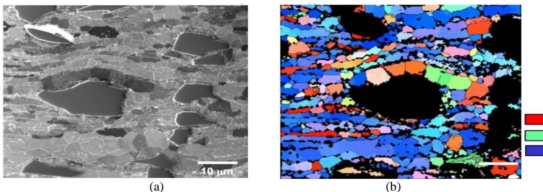
Fig 6: Microstructure of SiC particle reinforced 2080 Al matrix composite after hot extrusion.
