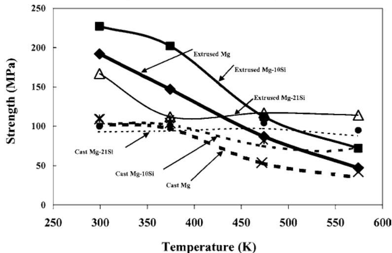
Fig 1: The tensile strength of the extruded and cast Mg-Si alloys [15]
