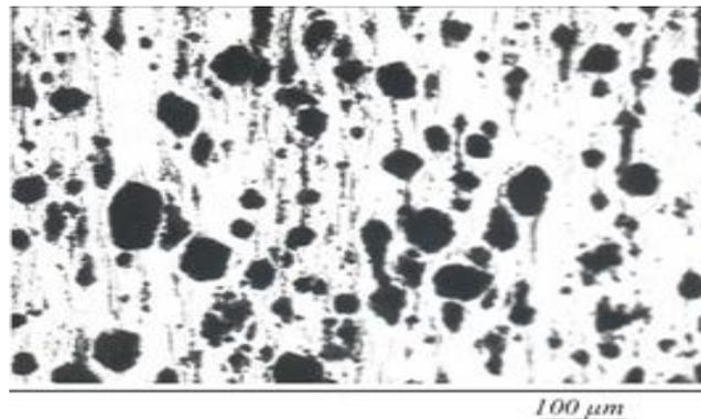
Fig 5: Microstructure of extruded 7475 Al -25 vol.%  $\text{Al}_2\text{O}_3$  particles(40  $\mu\text{m}$ ) [14]
