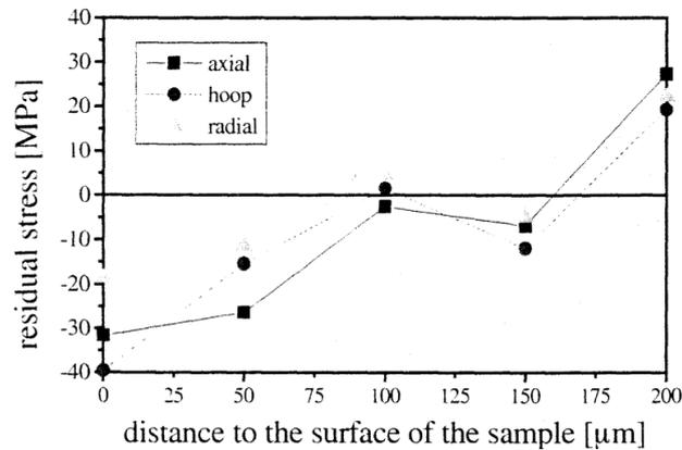
Fig 10: Residual stress in Al- matrix at 400°C [13]
