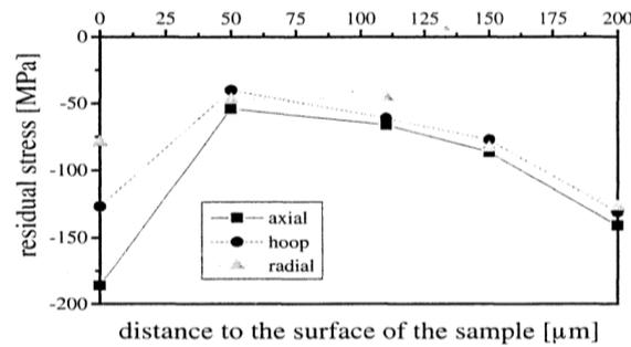
Fig 9: Residual stress in Si-particles, at 450°C [13]
