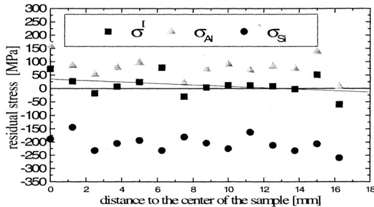
Fig 8: Residual stress in axial direction in the sample extruded at 450° C [13]
