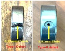
Figure 6.The Type-I and Type-II defect bearing
