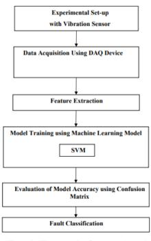
Figure 2. Flow graph of proposed work
