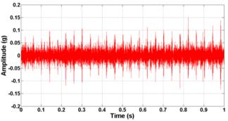
Figure 9. Vibration signal from type-II defect bearing
