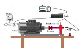
Figure 3. Schematic of the experimental setup
