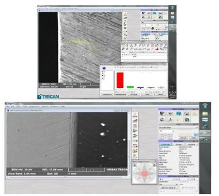
Figure 4. SEM and EDX images of Ni-plated samples within 18 minutes
