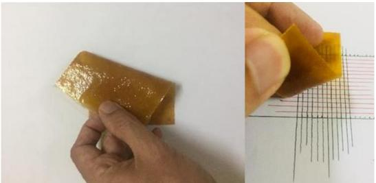
Figure 6. Adhesion test
