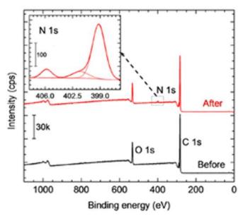
Figure 2. XPS survey spectra of pristine Plexiglas® before (black) and after (red) functionalization through nitrophenyl-vinylpyridine organic layer with the inset showing high resolution N 1s spectrum of the functionalized Plexiglas.
