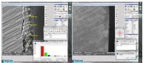
Figure 3. SEM and EDX images of Ni-plated samples within 09 minutes
