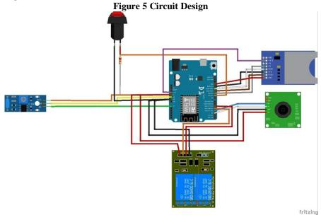
This design is made using the fritzing application, based on the block diagram that has been made so that there are no errors when the program is planted, while the pin installation circuit is described in the table below
