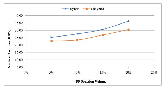
Figure 2. The suface hardnessof specimens
