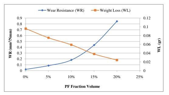
Figure 3. The wear resistance and weight loss of specimens
