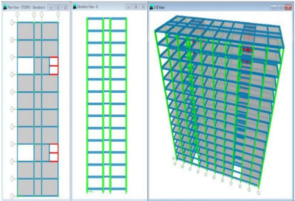
Figure 2. Building structure model in ETABS
