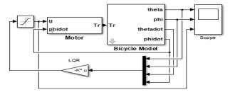
Figure 2. The scheme of LQR controller
