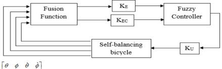
**Figure 3.** The model of fuzzy-LQR controller
