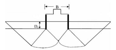
Figure 1. Increase in length of slip lines due to using of ring
