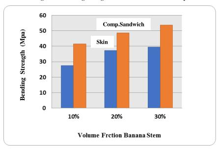
Figure 4. Bending strength of skin and sandwich composites
